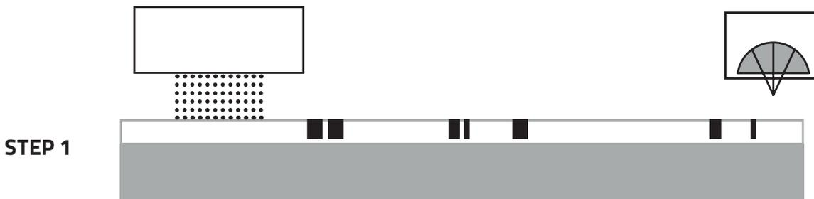
The texture is digitally printed into the wear layer. Texture and wear layer are cured.
